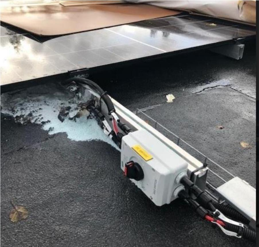
Figure 12: Burned isolator switch, 2022, licenced and approved by NÄRF.
