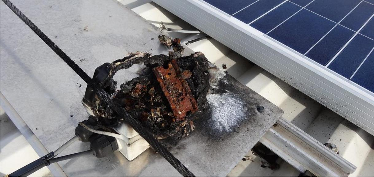
Figure 11: Burnt out isolator on the 300kw roof, h080, 2016, [solar panel failure | burnt out isolator on the 300kw roof | h080 | Flickr](#), CC BY-SA 2.0.
